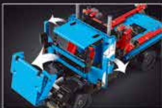
Open both doors and front hood 打开两侧车门和前车盖
